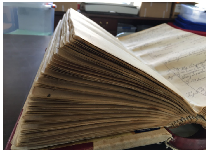
Sussex County Guardians Accounts, 1754-1789, was cellulose acetate laminated in 1939 and the pages are chipping and breaking, stiff, splitting and warping, with heavy burn through.
