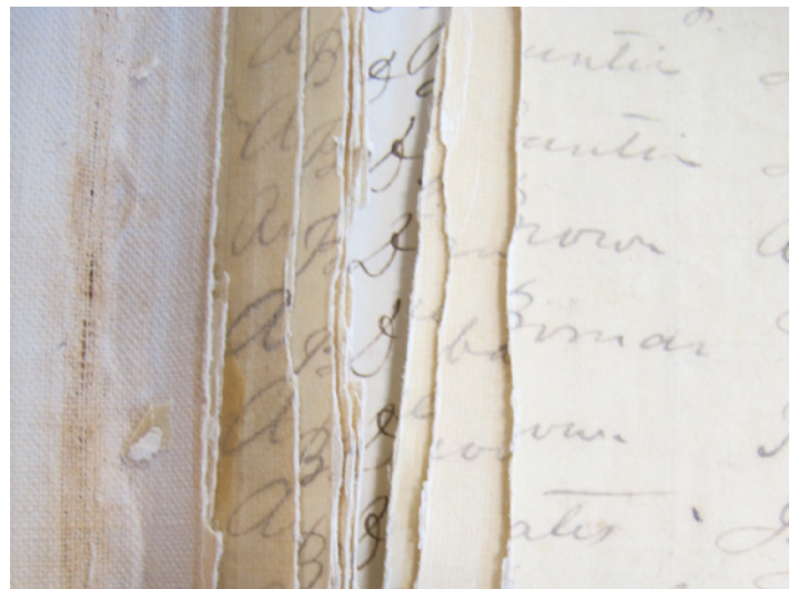
The cellulose acetate laminated pages in Halifax County Land Book, 1867-1872, have dried up and are beginning to break along the gutter.
